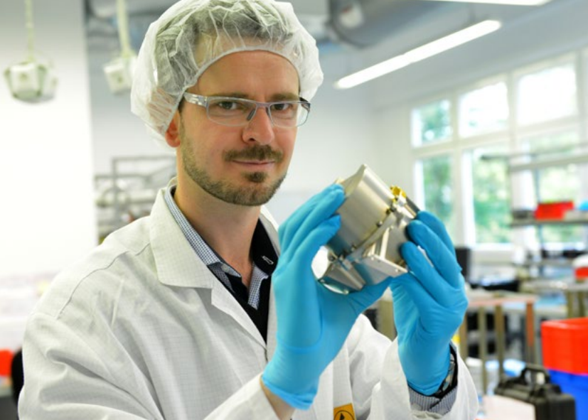
Engineer Sebastian Scheiding, managing director of Astro- und Feinwerktechnik Adlershof GmbH, with "RW90," a reaction wheel for satellites
