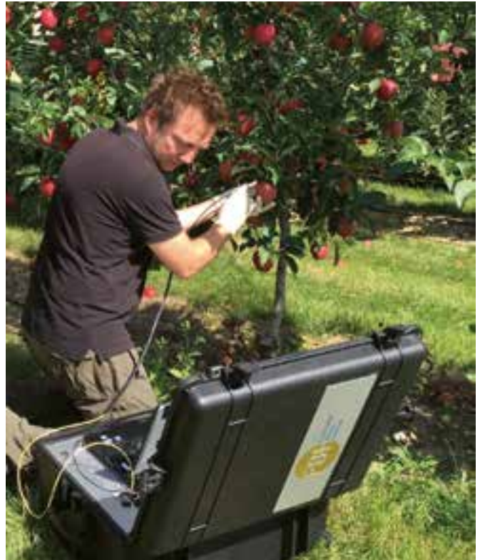
A portable Raman laser system for field use was developed at FBH, seen here in an orchard.
