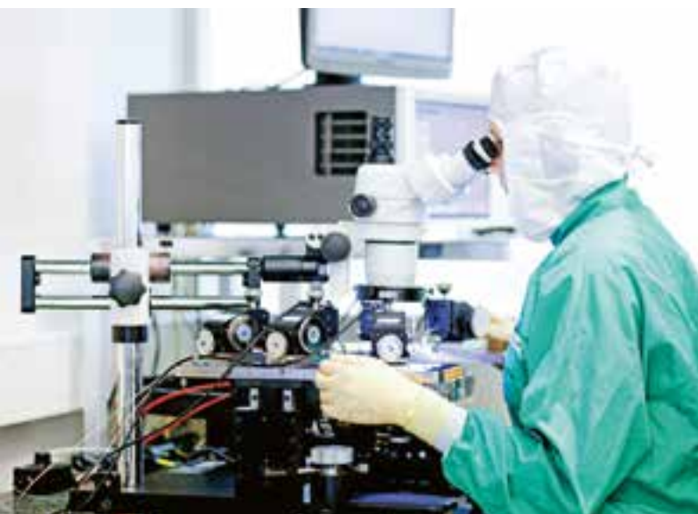
On-wafer chip characterisation at Fraunhofer HHI © Berlin Partner for Business and Technology – Monique Wüstenhagen
