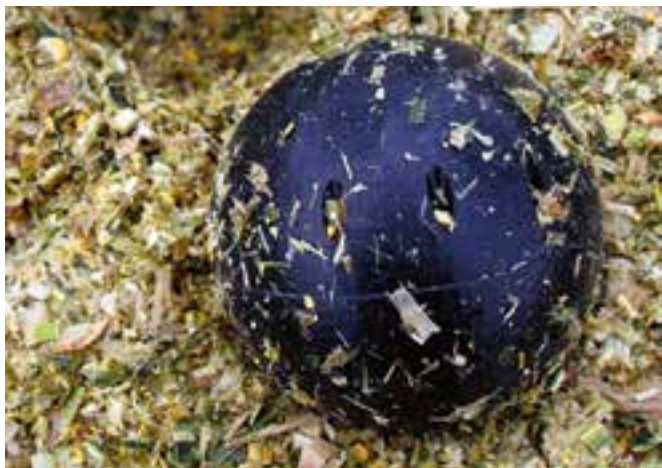
Sensor system for monitoring the ensiling process in biogas production © Fraunhofer IZM
