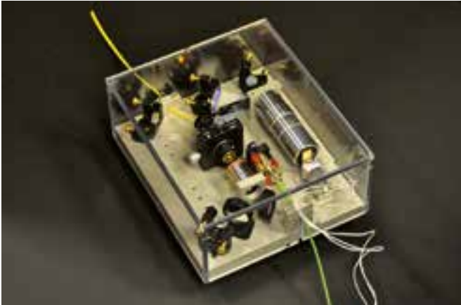
Single photon source for quantum experiments © AG Benson, HU Berlin
