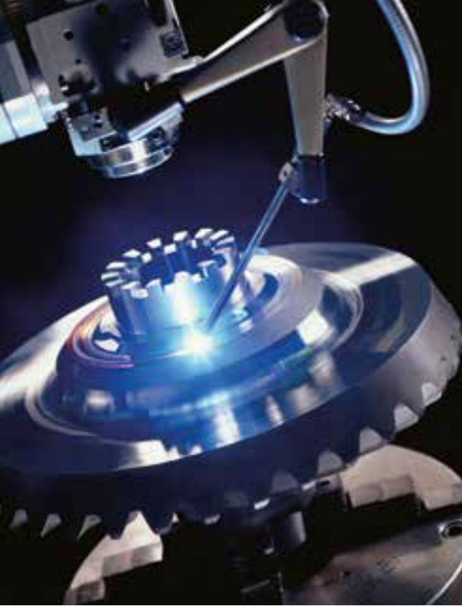
CO 2 lasers can produce slender and deep weld seams that withstand the highest mechanical loads.
