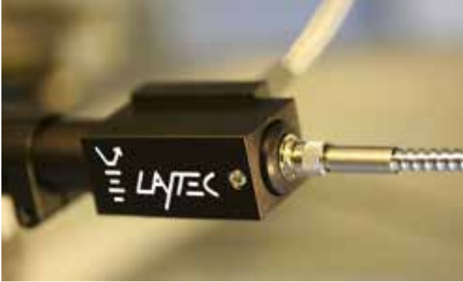
EpiTT in situ sensor to analyse growth during MOCVD and MBE processes © LayTec AG
