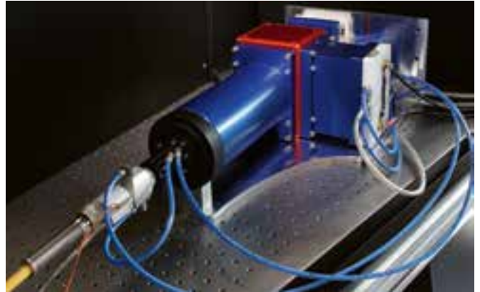
Pump module for high-energy short pulse laser systems with approx. 6 kW output power from the fibre
