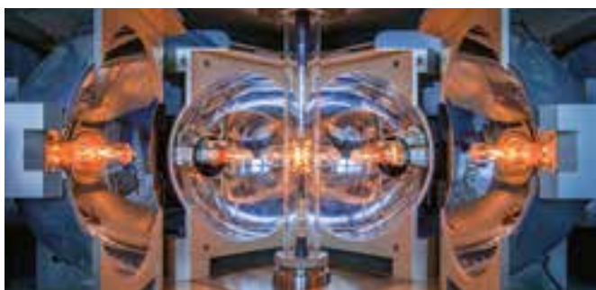
Large single crystals are produced in this optical zone melting furnace. © M. Setzpfandt/HZB
