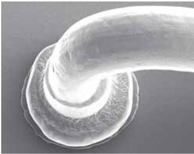
Ball bond contact on a high-strength aluminium scandium (AlSc) chip metallisation
