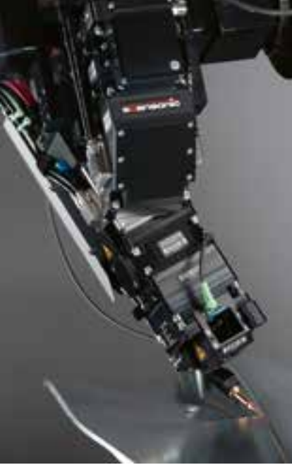
ALO3: laser processing optics with seam tracking by added wire © Scansonic Group
