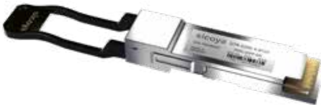
Optical transceiver module for data centre connections © Sicoya GmbH
