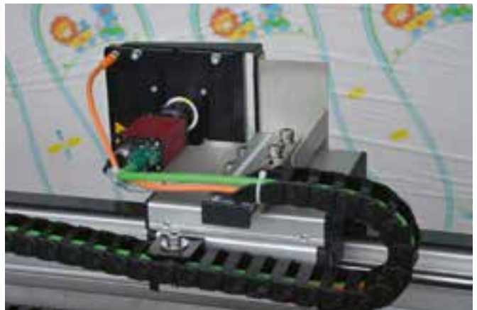
Camera on axis in front of a printing web © Bi-Ber GmbH & Co. Engineering KG
